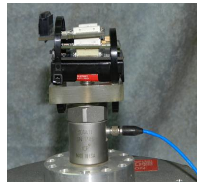
Fig. 6 Imote Sensor Mounted in the Vibration Test Bench
